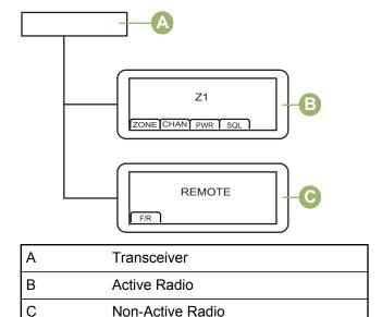
You can change the command between the 2 control heads by pressing the **Menu Select** button directly below F/R, or the **Menu Select** button preprogrammed user button on the keypad microphone.
